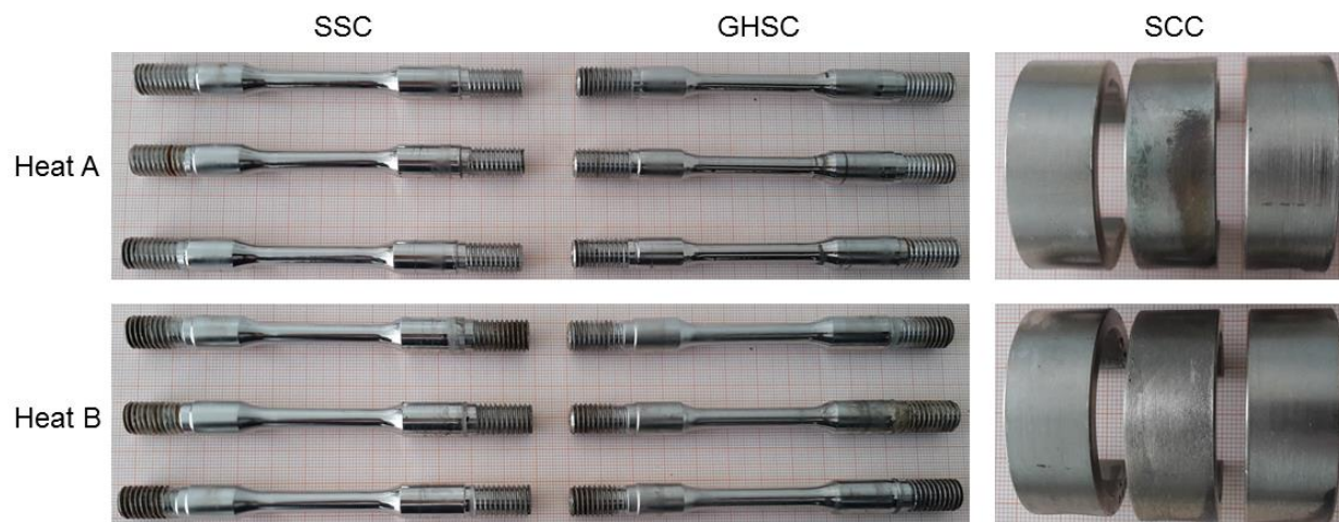
Figure 6: SSC and GHSC specimens after test according to NACE TM0177 Method A, for 30 days; SCC specimens according to NACE TM0177 Method C at Level VII condition for 30 days
